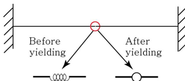
Fig. 1 Implementation of rotational spring elements
